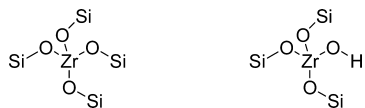
Chart 2. Configurations of Closed (left) and Open (right) Sites of the ZrBEA Zeolite
